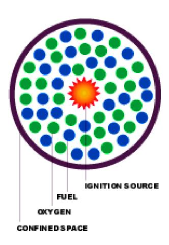
Why does an explosion occur? In order for a deflagration explosion to occur four elements are required. These are; Fuel, Oxygen, An ignition source and a confined space.
