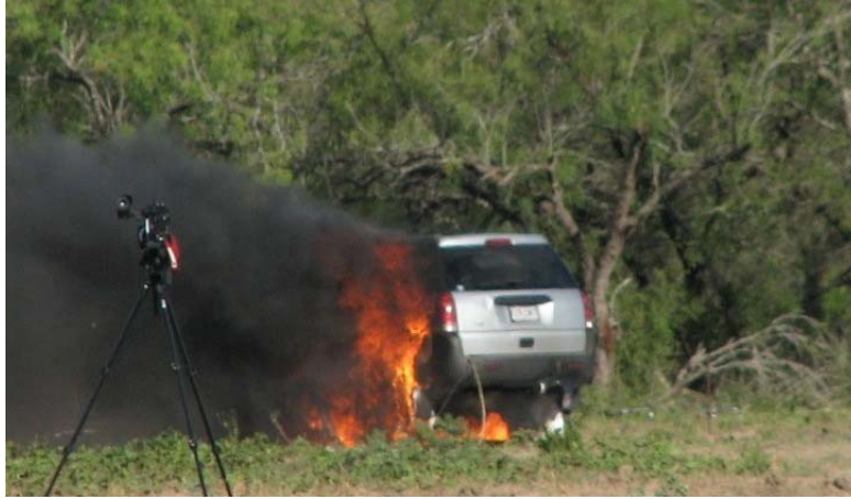
Figure 11 Fire 9 minutes after ignition under hydrogen cylinder (from Zalosh)
