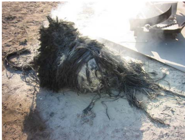
Figure 12b Type 3 hydrogen cylinder fragment (from Zalosh)
