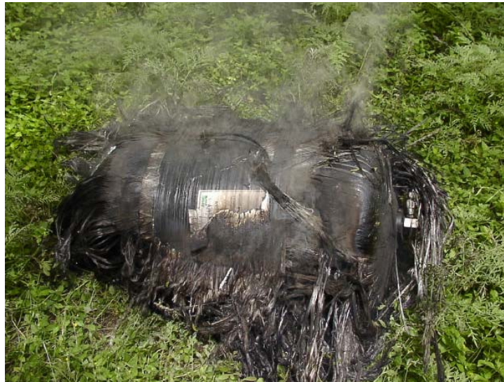
Figure 12a Type 4 hydrogen cylinder fragment (from Zalosh)
