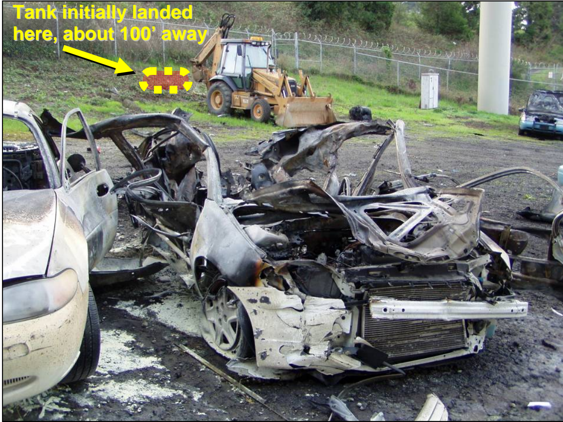
Figure 6. Remains of Honda CNG vehicle from March 2007 fire in Seattle.
