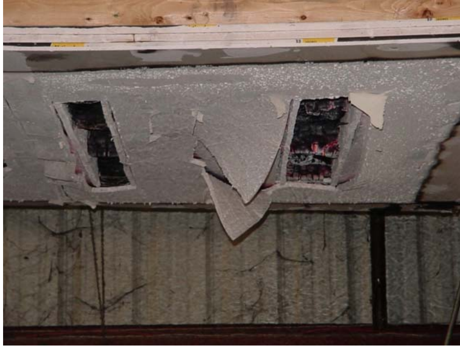
Removing the assembly from the furnace
