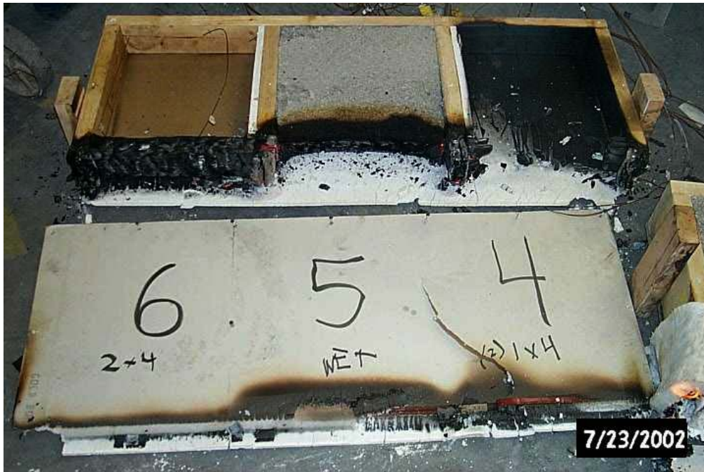
Approximately 10" of virgin material remained in the insulated cavity, the 2 x 4 was charred, and the two 1 x 4 were completely burnt
