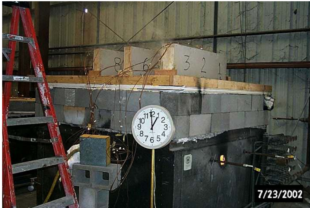
The furnace was extinguished after 60 minutes
