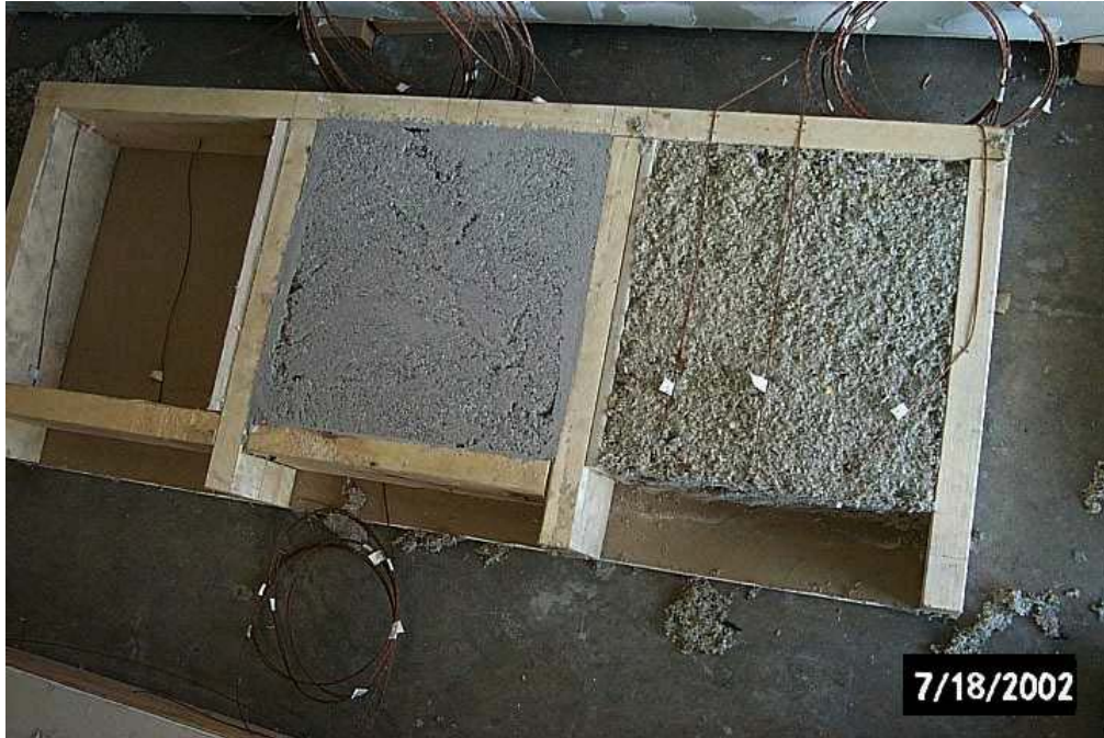
(L-R) single 2 x 4, dry-fill insulation, wet spray insulation (the block in the center cavity was removed prior to testing)
