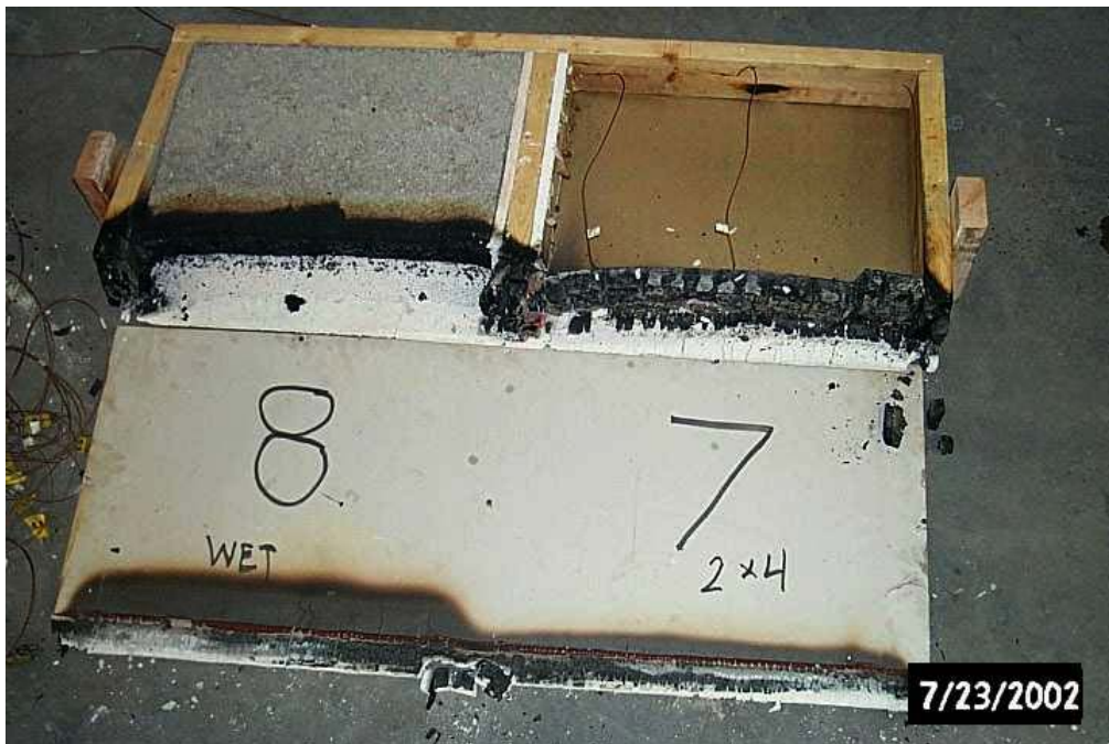
Approximately 10" of virgin material remained in the insulated cavity, the 2 x 6 was charred
